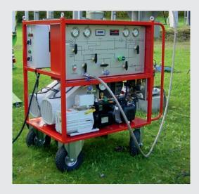
For maintenance of gas insulated switchgear, portable recovery units are used, consisting of one or more vacuum pumps, a filter and a HAUG Sauer compressor.
